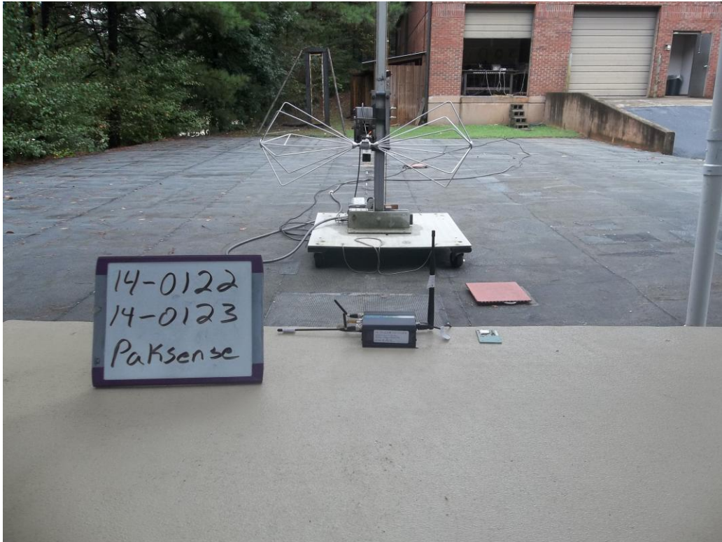
Photo 4- Radiated Emissions Test Setup, 30 MHz to 200 MHz, Back
