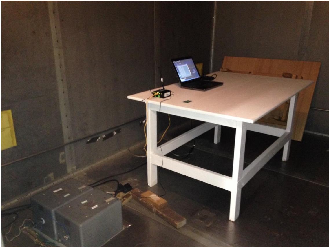
Photo 9- Conducted Emissions Test Setup, with RF Label
