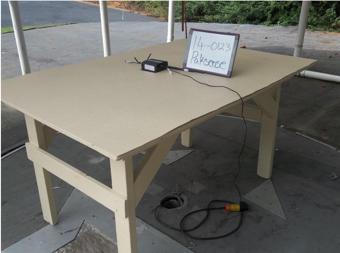
Photo 2- Radiated Emissions Test Setup, Front, without RF Label
