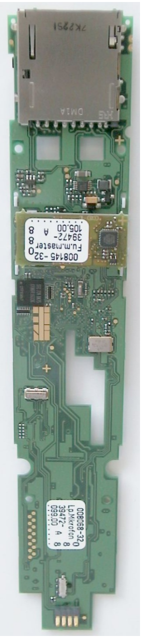
Digta CordEx Microphone PCB bottem side with wireless-modul
