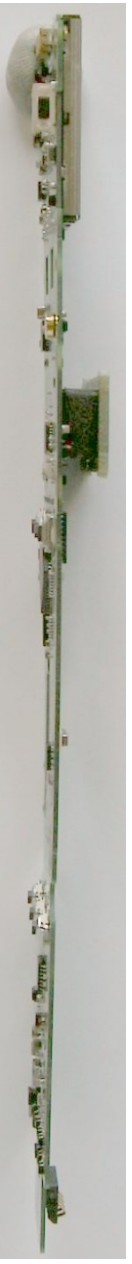
Digta CordEx Microphone PCB right side with wireless-modul
