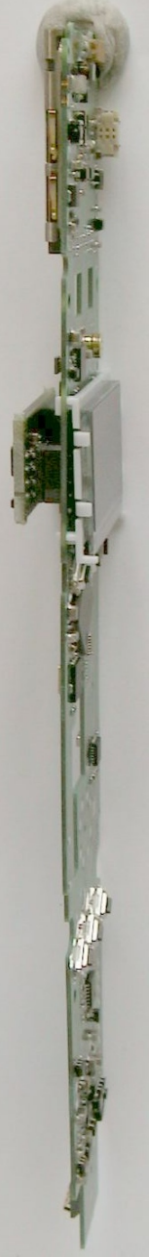
Digita CordEx Microphone PCB left side with wireless-modul and display
