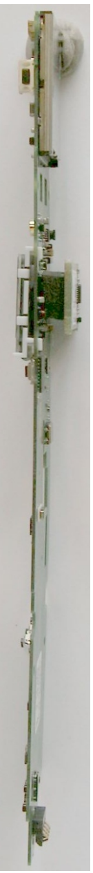
Digta CordEx Microphone PCB right side with wireless-modul and display
