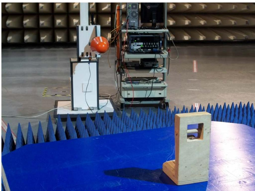
Worst case set-up for radiated emission test above 1 GHz distance 3m
