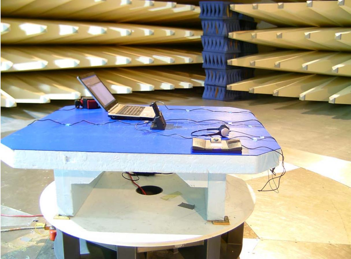
Worst case set-up for radiated emission; 30 MHz - 1 GHz distance 10m
