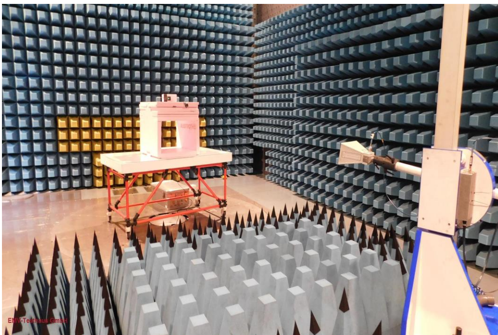
Picture 8: SAC, radiated emission test 1 GHz – 18 GHz and band-edge– position Z (back view)
