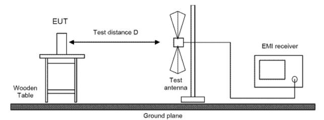
Picture 5: Test setup for radiated emission measurement (< 1 GHz)
