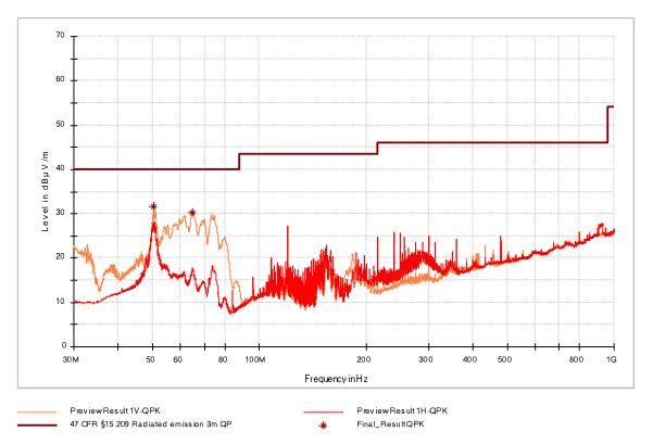
Picture 8: Radiated emission 30 MHz - 1000MHz @ 3m distance
