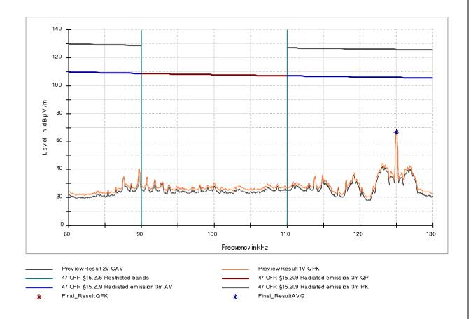
Picture 7: Restricted band of operation, PK / AV @ 3m distance
