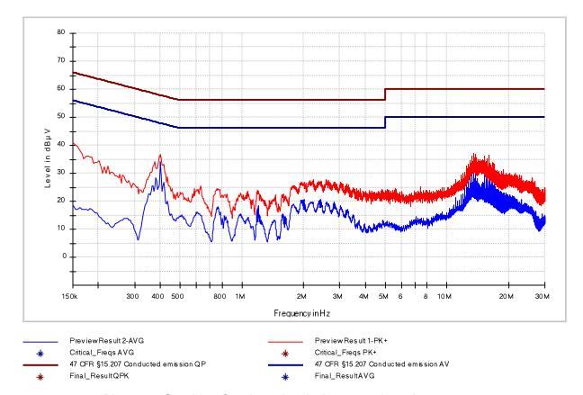
Picture 2: Graphic - Conducted emission on mains, phase 1
