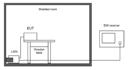
Picture 1: Outline of conducted emission test setup
