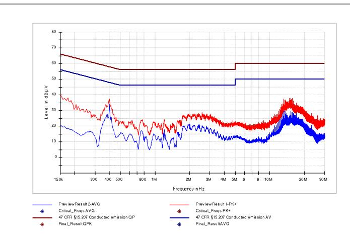
Picture 3: Graphic - Conducted emission on mains, neutral
