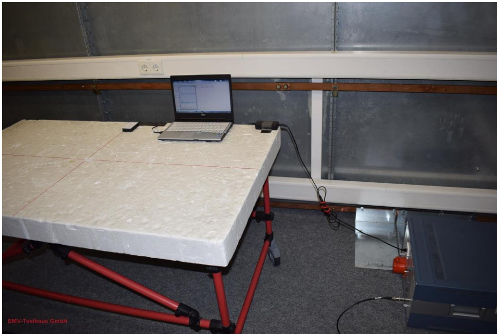
Picture 3: Test setup AC power line conducted emissions (front view)
