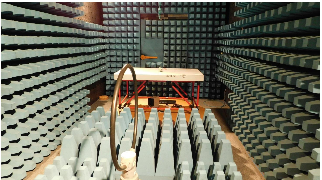
Picture 2: CDC, test setup radiated emission test 9 kHz -30 MHz (rear view)
