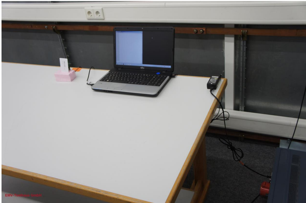
Picture 6: Test setup AC power line conducted emissions (front view)
