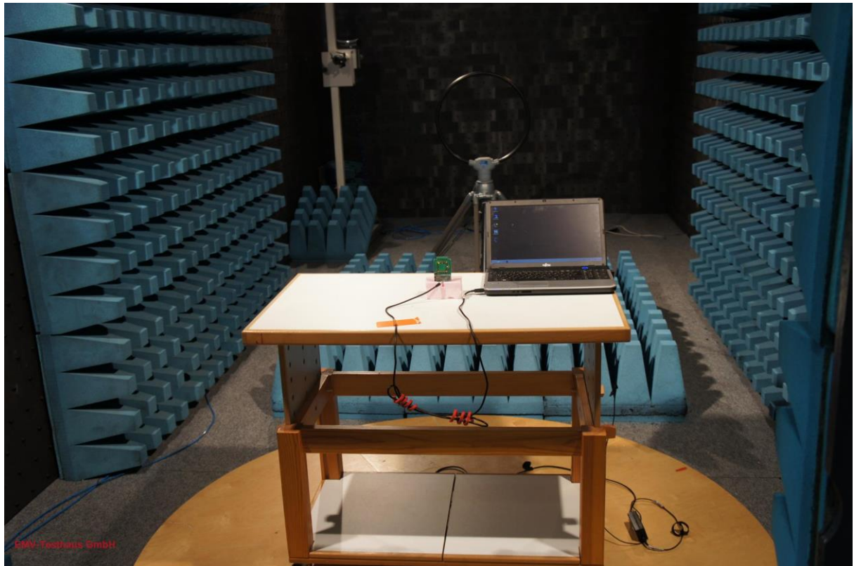
Picture 1: CDC, test setup radiated emission test 9 kHz -30 MHz (front view)
