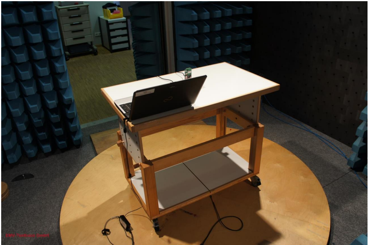
Picture 3: CDC, test setup radiated emission test (rear view)
