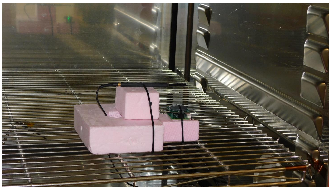
Picture 10: Carrier frequency test in climate chamber
