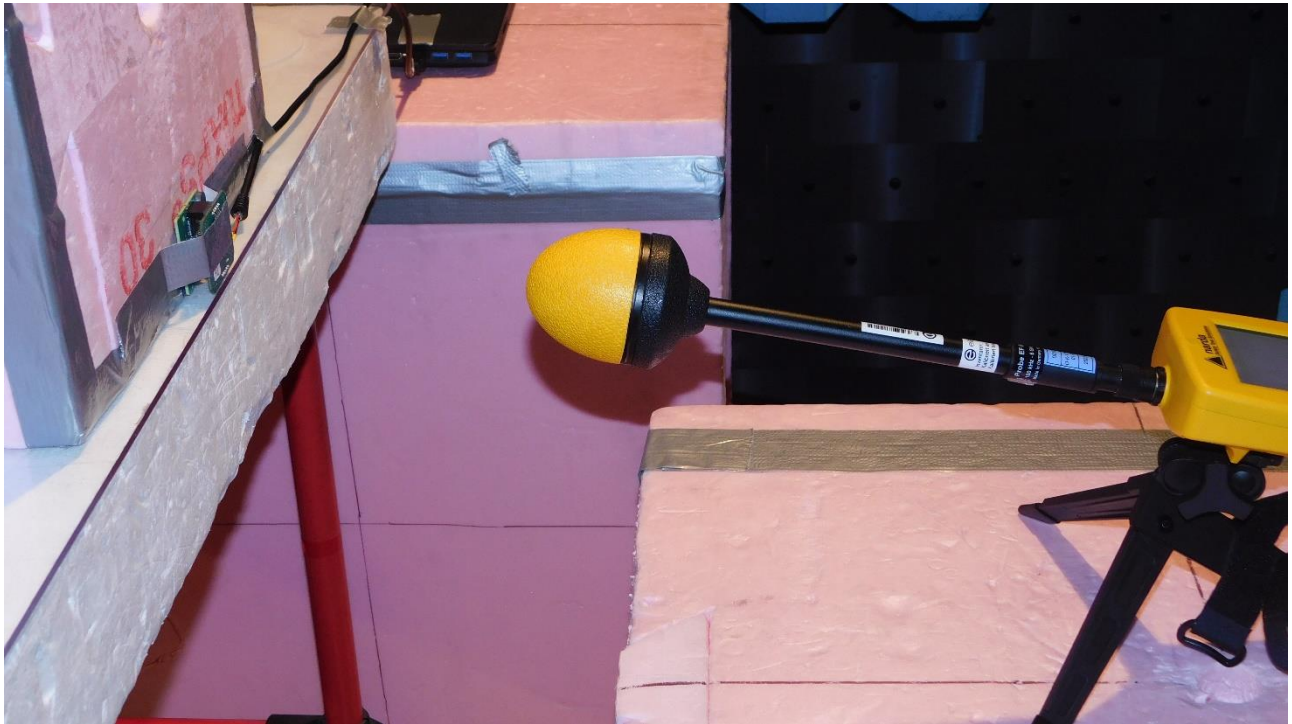
Picture 2: Setup of electric field test at a measurement distance of 20 cm, without RFID tag
