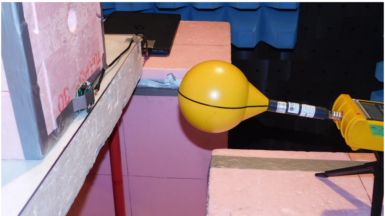
Picture 1: Setup of magnetic field test at a measurement distance of 20 cm, without RFID tag
