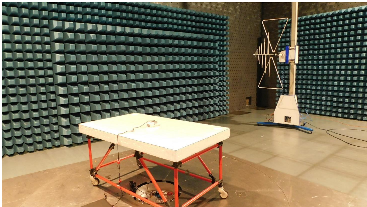
Picture 3: SAC, radiated emission test 30 MHz -1 GHz (front view)
