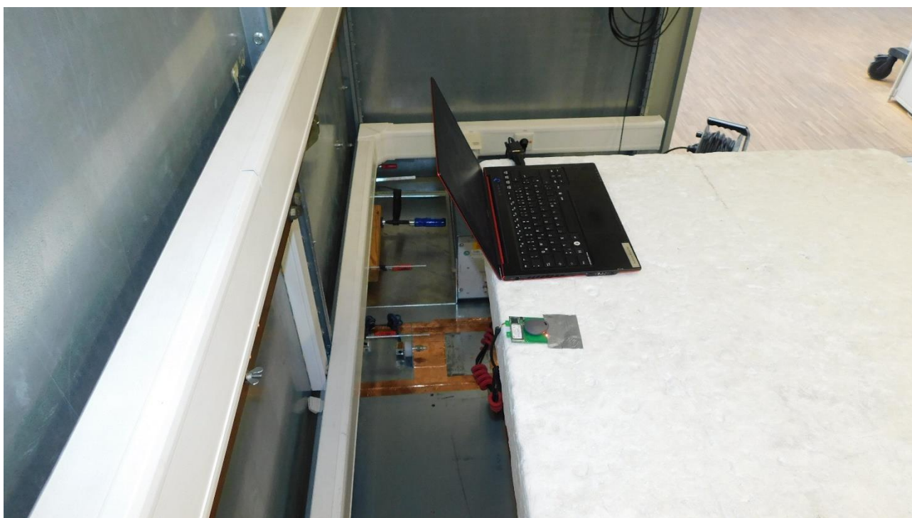
Picture 10: Test setup AC power line conducted emissions (rear view), RS232
