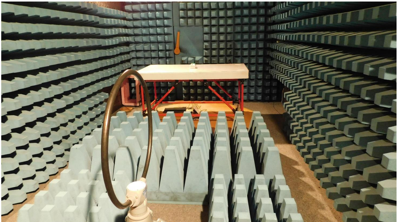
Picture 2: CDC, test setup radiated emission test 9 kHz -30 MHz and bandwidth measurement (rear view)
