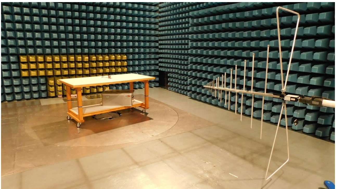
Picture 4: SAC, radiated emission test 30 MHz -1 GHz (rear view)
