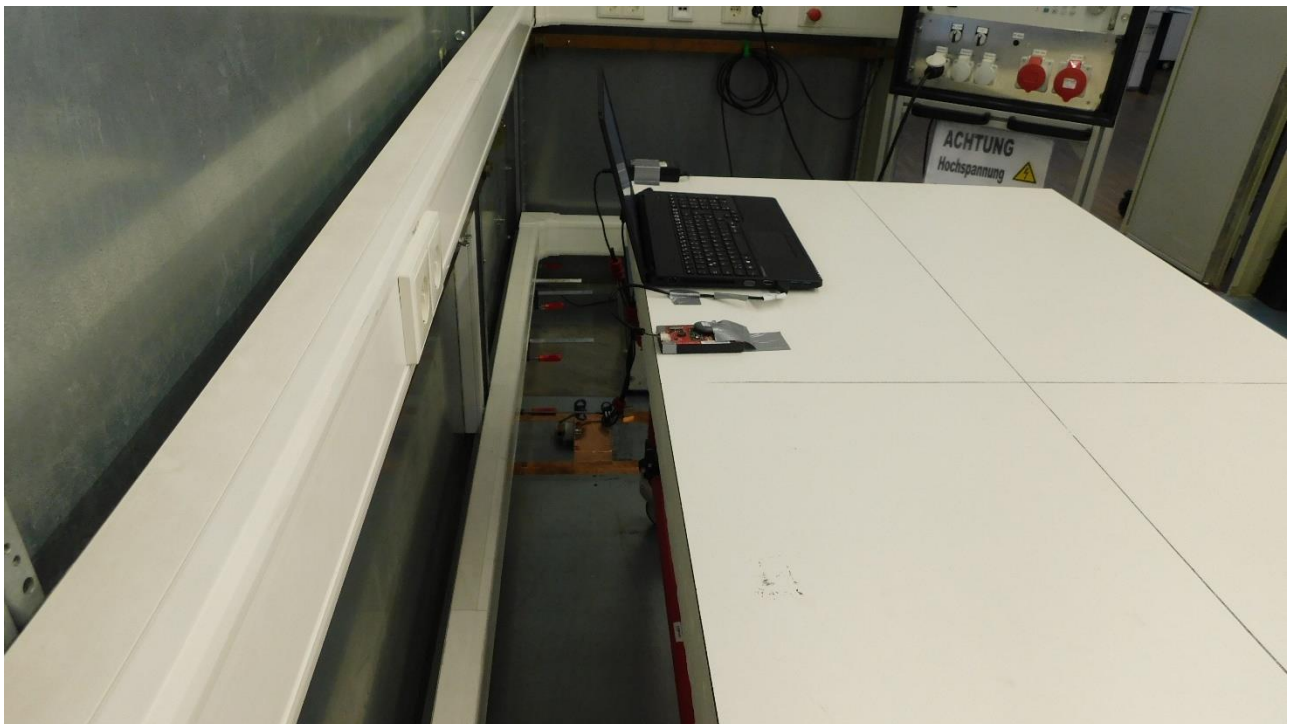
Picture 8: Test setup AC power line conducted emissions (rear view), USB
