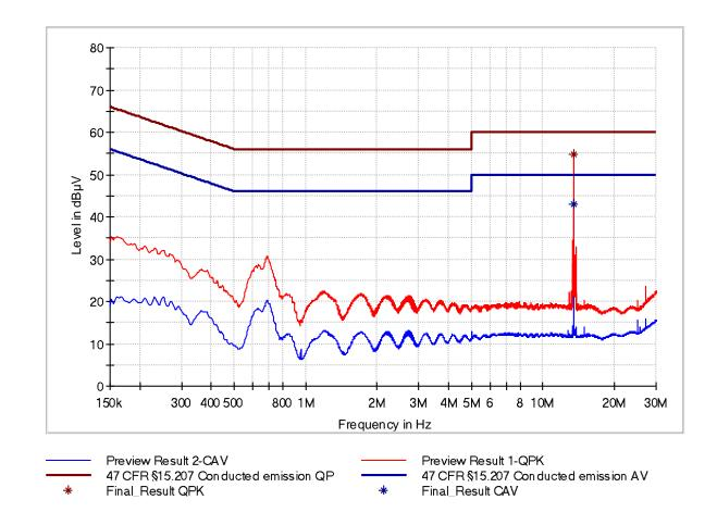
Figure 9: Chart of AC power-line conducted emissions test – phase N, RS232
