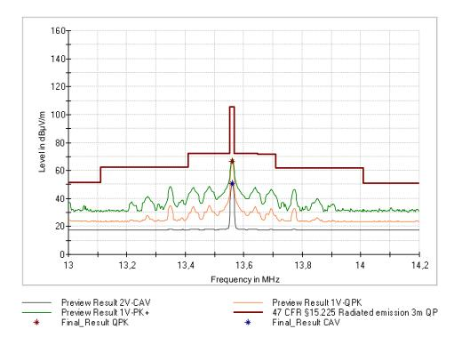
Figure 15: Chart of emission within the band 13.110 MHz to 14.010 MHz, EUT in position Z, without tag, antenna in line at 3 m distance, RS232
