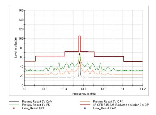
Figure 14: Chart of emission within the band 13.110 MHz to 14.010 MHz, EUT in position Z, without tag, antenna in line at 3 m distance, USB
