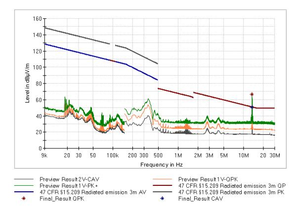
Figure 17: Chart of emissions test below 30 MHz, EUT position Z, without tag, antenna in line at 3 m, RS232
