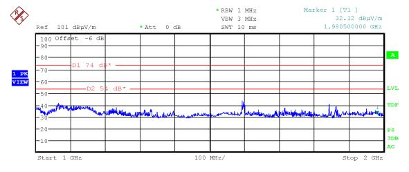
Figure 21: Chart of emissions test from 1 GHz to 2 GHz, EUT position Y, without tag, antenna vertical, at 3 m, RS232
