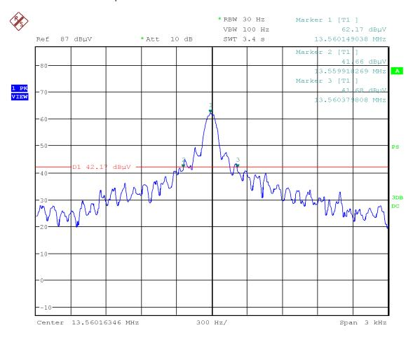
Figure 11: Chart of 20 dB bandwidth tests, with tag, RS232
