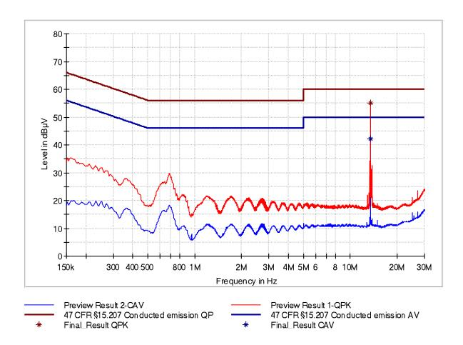
Figure 8: Chart of AC power-line conducted emissions test – phase L1, RS232
