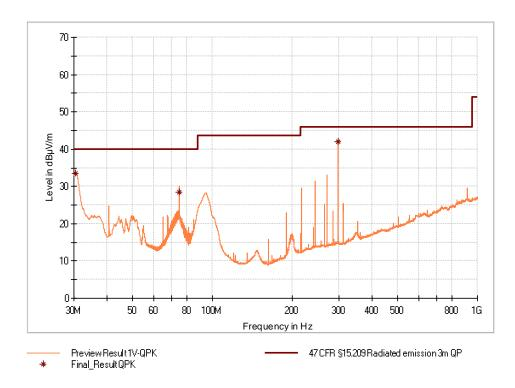
Figure 19: Chart of emissions test from 30 MHz to 1 GHz, EUT position Z, without tag, antenna vertical, at 3 m, RS232
