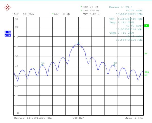
Figure 13: Chart of occupied bandwidth test, without tag, RS232
