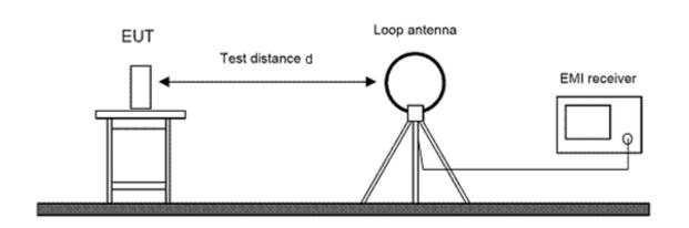
Figure 2: Setup for radiated emissions test below 30 MHz
