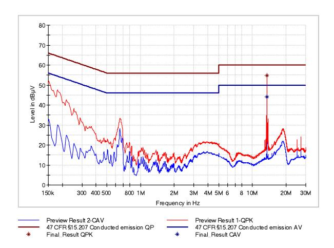
Figure 6: Chart of AC power-line conducted emissions test - phase L1, USB
