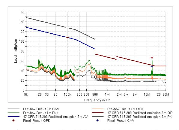
Figure 16: Chart of emissions test below 30 MHz, EUT position Z, without tag, antenna in line at 3 m, USB
