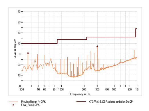
Figure 18: Chart of emissions test from 30 MHz to 1 GHz, EUT position Z, without tag, antenna vertical, at 3 m, USB
