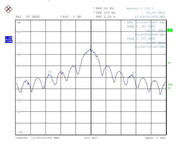
Figure 12: Chart of occupied bandwidth test, without tag, USB
