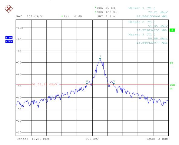
Figure 10: Chart of 20 dB bandwidth tests, with tag, USB
