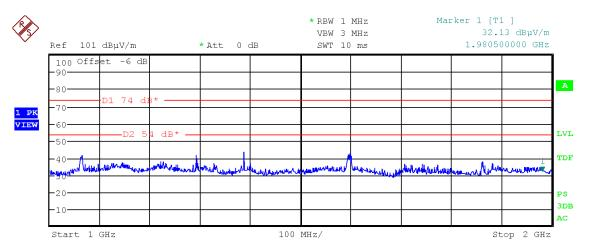
Figure 20: Chart of emissions test from 1 GHz to 2 GHz, EUT position Y, without tag, antenna vertical, at 3 m, USB
