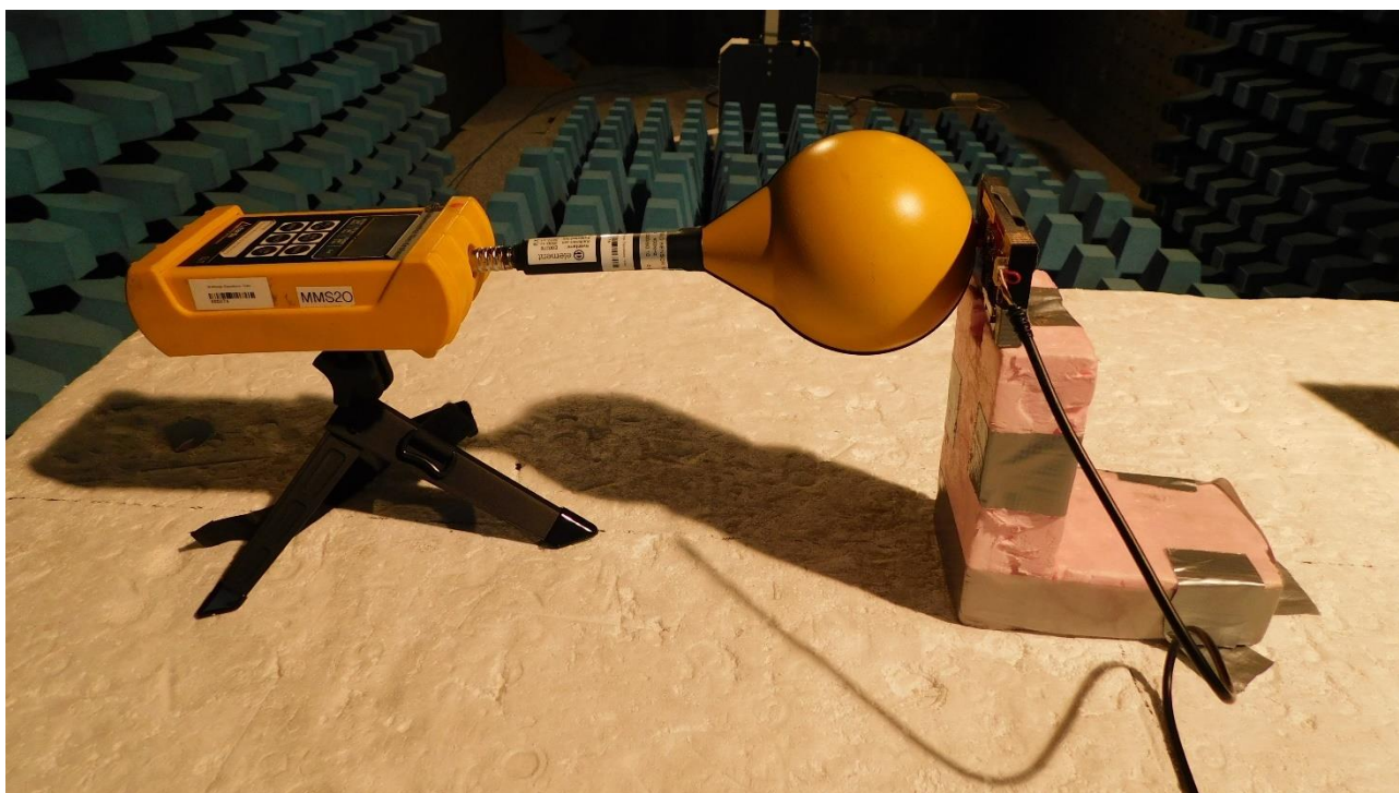
Picture 1: Setup of magnetic field test at a measurement distance of 0 cm
