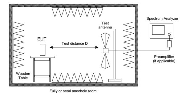
Figure 4: Setup for radiated emissions test above 1 GHz
