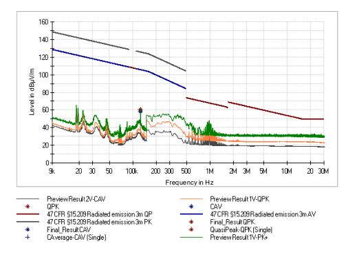
Figure 14: Chart of emissions test below 30 MHz, EUT position Z, without tag, antenna parallel at 3 m, RS232
