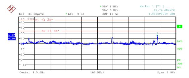
Figure 18: Chart of emissions test from 1 GHz to 2 GHz, EUT position X, with tag, antenna vertical, RS232
