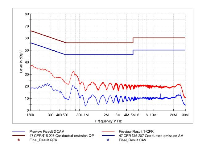
Figure 10: Chart of AC power-line conducted emissions test – phase N, RS232
