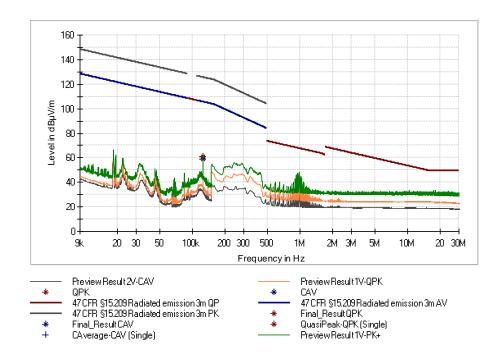
Figure 13: Chart of emissions test below 30 MHz, EUT position Y, without tag, antenna parallel at 3 m, USB
