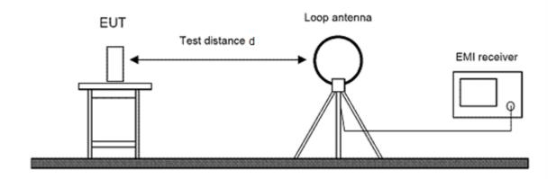
Figure 2: Setup for radiated emissions test below 30 MHz
