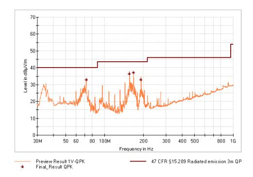
Figure 16: Chart of emissions test from 30 MHz to 1 GHz, EUT position Y, with tag, antenna vertical, at 3 m, RS232
