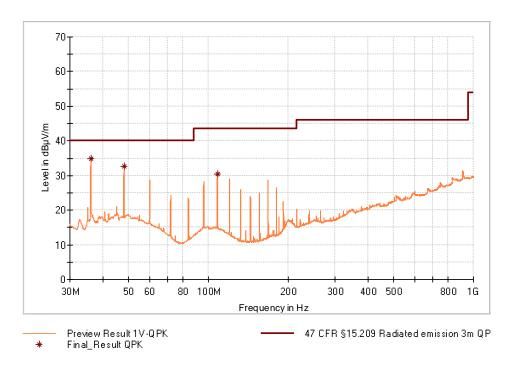
Figure 15: Chart of emissions test from 30 MHz to 1 GHz, EUT position Y, with tag, antenna vertical, at 3 m, USB
