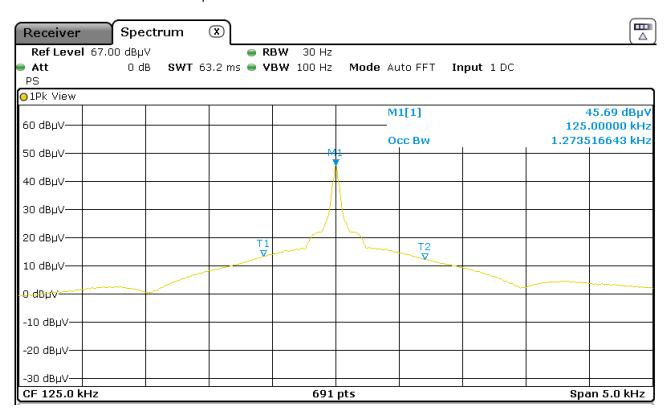
Figure 12: Chart of occupied bandwidth test, with tag, RS232
