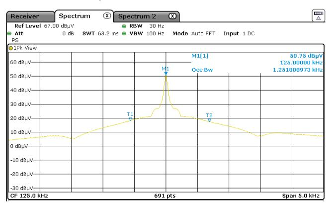
Figure 11: Chart of occupied bandwidth test, without tag, USB
