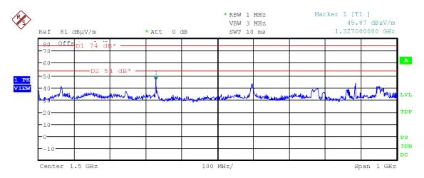
Figure 17: Chart of emissions test from 1 GHz to 2 GHz, EUT position X, with tag, antenna vertical, USB
