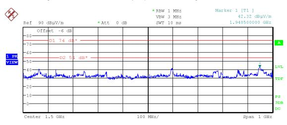
Figure 24: Chart of emissions test from 1 GHz to 2 GHz, EUT position X, with tag, antenna vertical, USB
