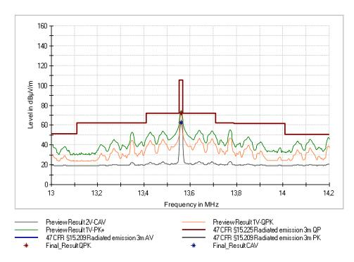
Figure 18: Chart of emission within the band 13.110 MHz to 14.010 MHz, EUT in position X, without tag, antenna in line at 3 m distance, USB
