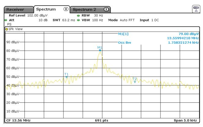
Figure 16: Chart of occupied bandwidth test, without tag, USB
