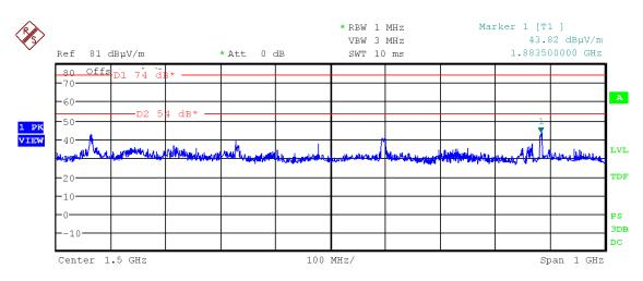
Figure 25: Chart of emissions test from 1 GHz to 2 GHz, EUT position X, with tag, antenna vertical, RS232
