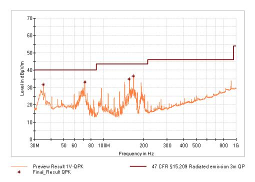
Figure 23: Chart of emissions test from 30 MHz to 1 GHz, EUT position Y, with tag, antenna vertical, at 3 m, RS232
