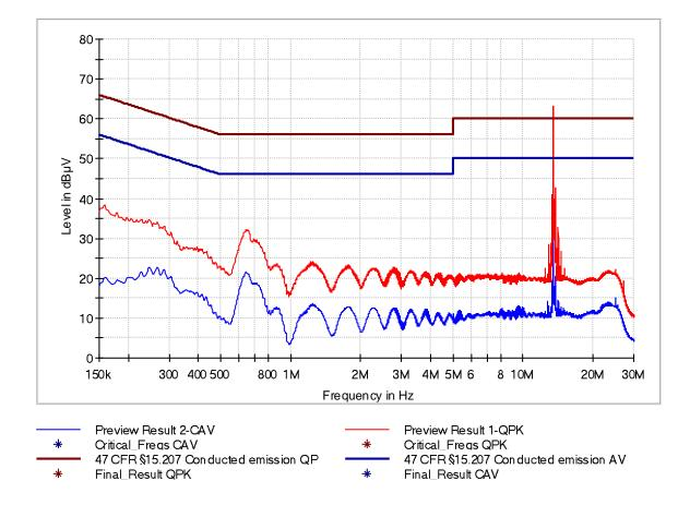
Figure 11: Chart of AC powerline conducted emissions on N – without termination, RS232
