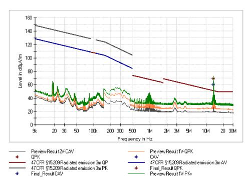
Figure 21: Chart of emissions test below 30 MHz, EUT position X, without tag, antenna in line at 3 m, RS232
