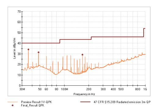
Figure 22: Chart of emissions test from 30 MHz to 1 GHz, EUT position Y, with tag, antenna vertical, at 3 m, USB
