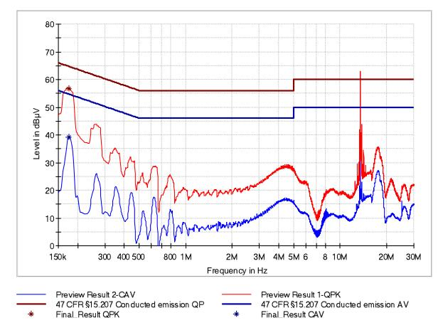
Figure 7: Chart of AC powerline conducted emissions on N - without termination, USB
