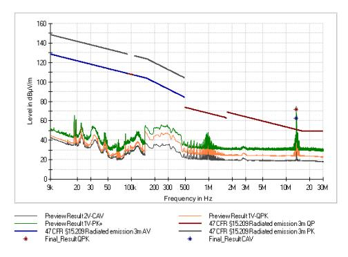
Figure 20: Chart of emissions test below 30 MHz, EUT position X, without tag, antenna in line at 3 m, USB
