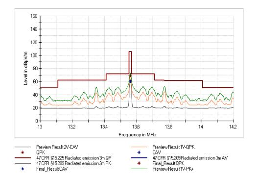
Figure 19: Chart of emission within the band 13.110 MHz to 14.010 MHz, EUT in position X, without tag, antenna in line at 3 m distance, RS232
