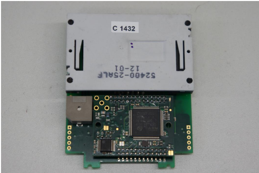
Picture 3: PCB bottom side (with card reader)
