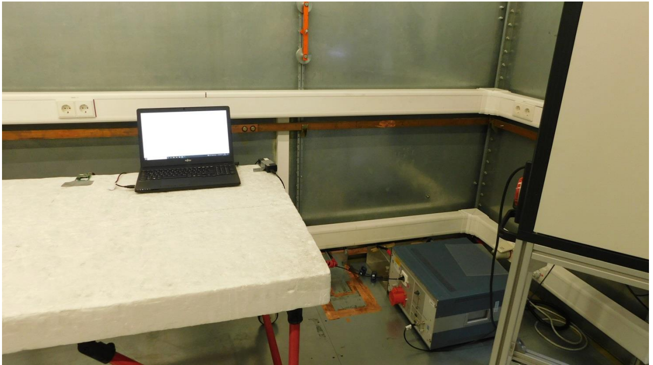
Picture 7: Test setup AC power line conducted emissions (front view)
