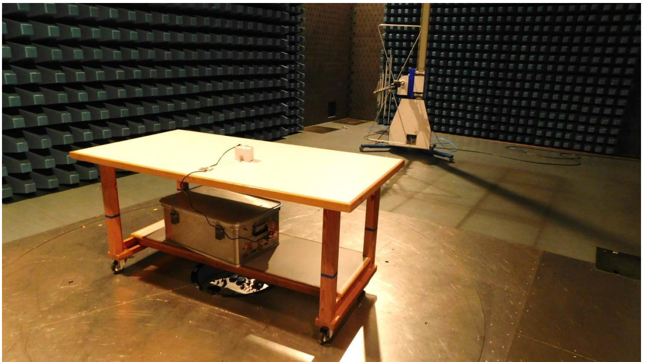
Picture 3: SAC, radiated emission test 30 MHz -1 GHz (front view)
