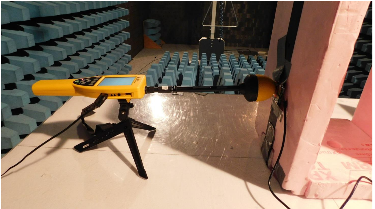
Picture 2: Setup of electric field test at a measurement distance of 0 cm
