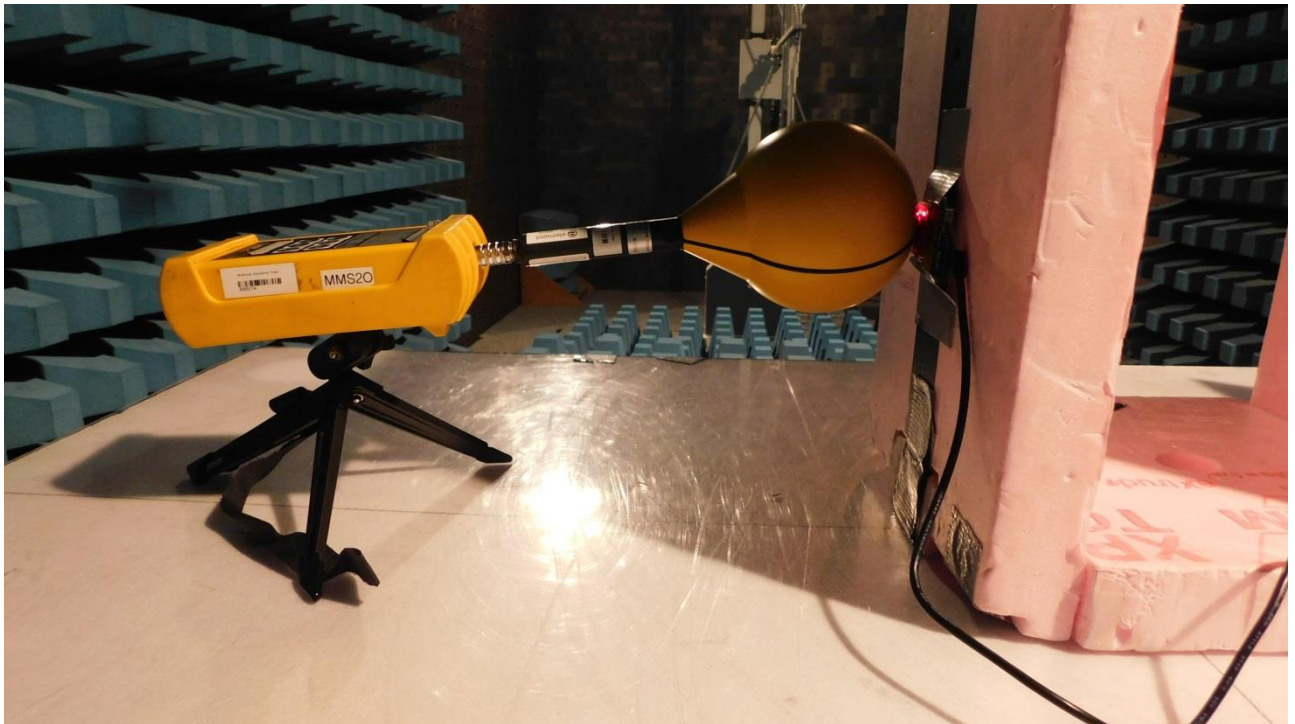
Picture 1: Setup of magnetic field test at a measurement distance of 0 cm
