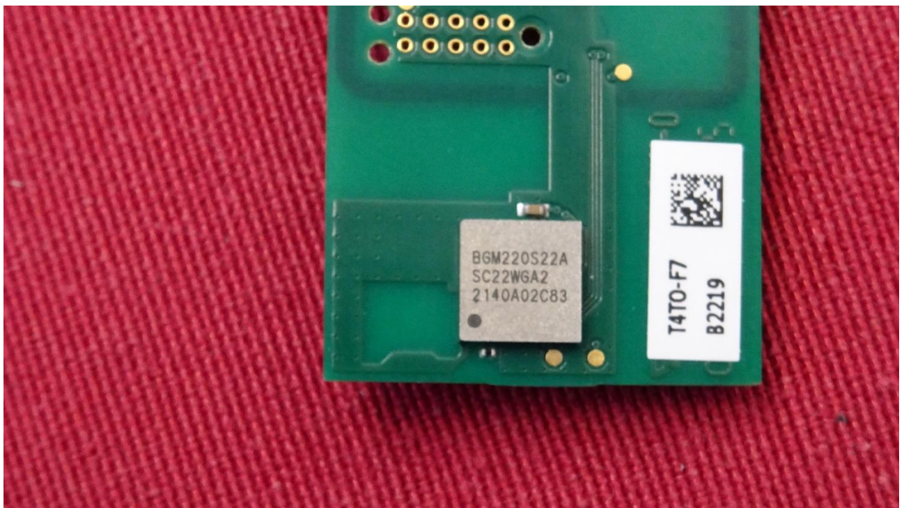
Picture 6: Name plate of BLE-chip
