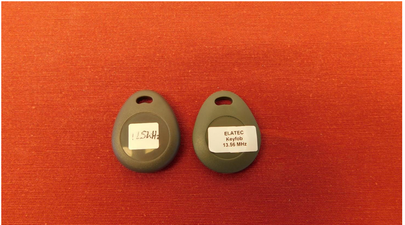
Picture 14: RFID tags 125 kHz and 13.56 MHz
