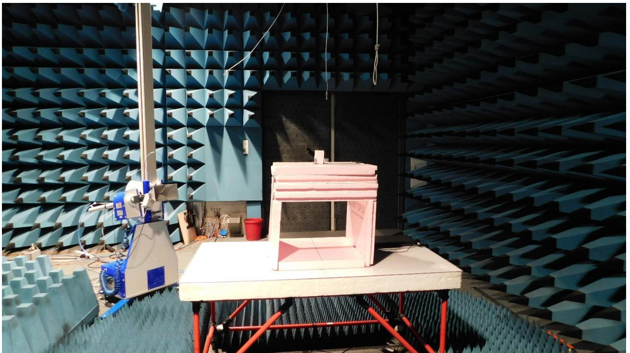
Picture 7: FS-SAC, radiated emission test 1 GHz – 17 GHz (rear view)
