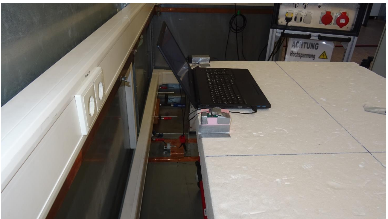
Picture 10: Test setup AC power line conducted emissions (rear view)
