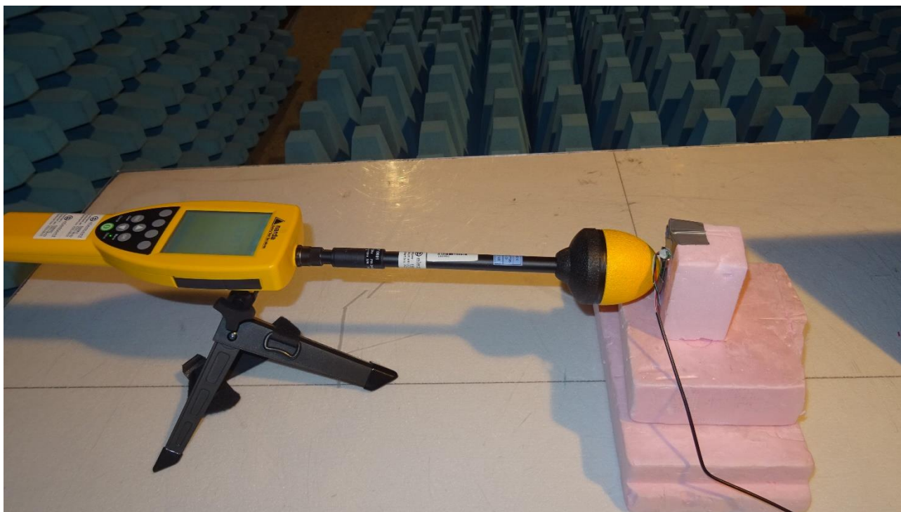
Picture 2: Setup of electric field test at a measurement distance of 0 cm
