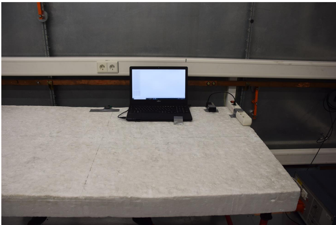
Picture 7: Test setup AC power line conducted emissions (front view)
