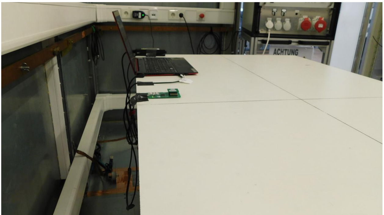
Picture 8: Test setup AC power line conducted emissions (rear view)
