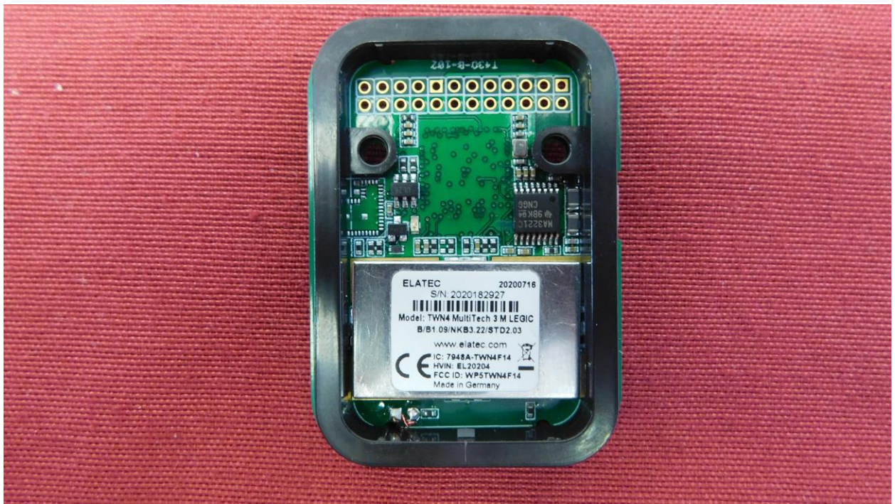
Picture 1: Top view of EUT with shielding
