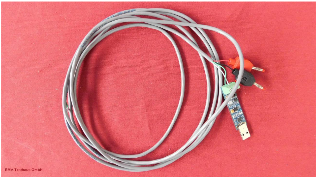
Picture 12: RS-485 adaptor + wiring
