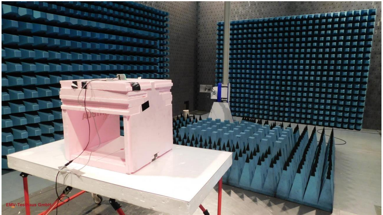
Picture 5: SAC, radiated emission test 1 GHz – 2 GHz (front view)
