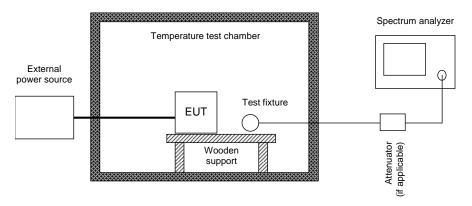
Figure 5: Test setup for carrier frequency stability measurement
