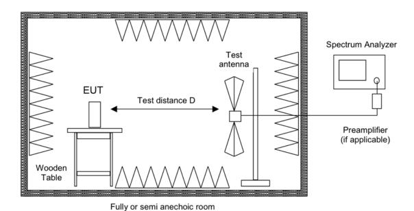
Figure 4: Setup for radiated emissions test above 1 GHz
