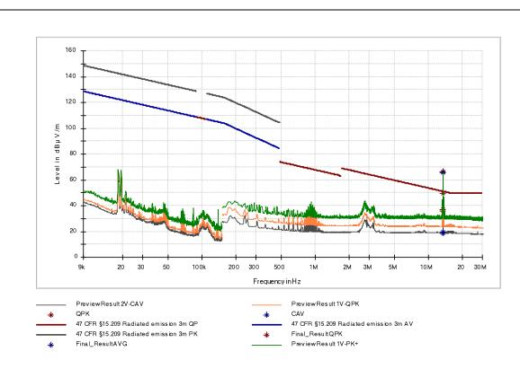
Figure 15: Chart of emissions test below 30 MHz without tag in position 2, antenna in line at 3 m, USB active
