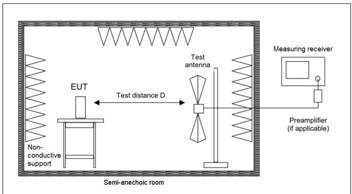
Figure 3: Setup for radiated emissions test from 30 MHz to 1 GHz
