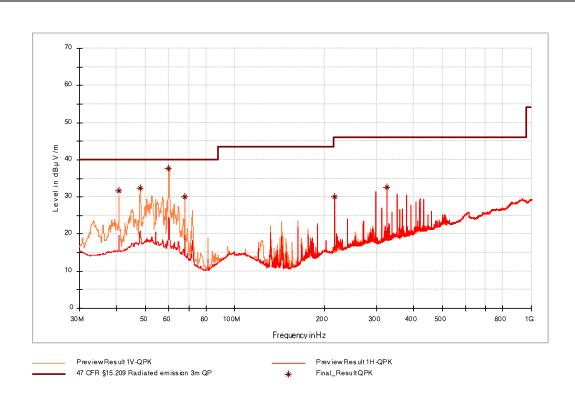
Figure 18: Chart of emissions test from 30 MHz to 1 GHz with tag in position 2 at 3 m, USB active
