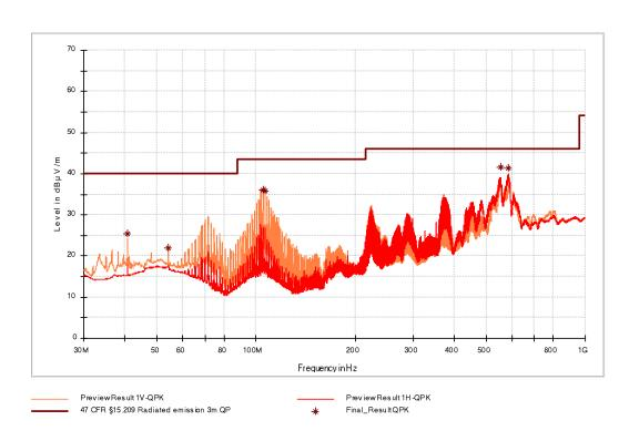
Figure 17: Chart of emissions test from 30 MHz to 1 GHz with tag in position 2 at 3 m, RS-232 active
