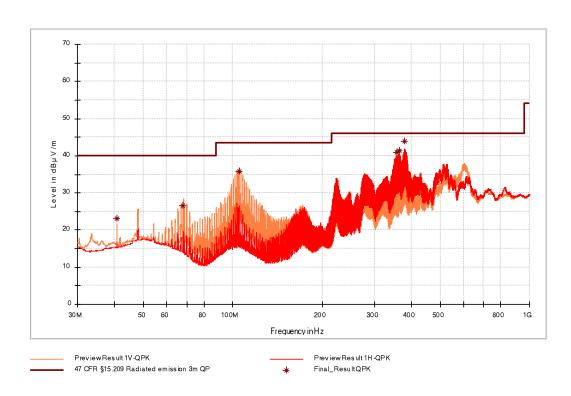
Figure 16: Chart of emissions test from 30 MHz to 1 GHz with tag in position 2 at 3 m, RS-485 active
