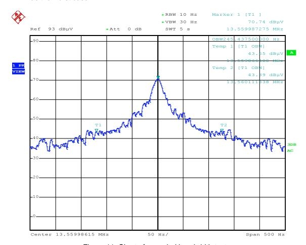
Figure 11: Chart of occupied bandwidth test
