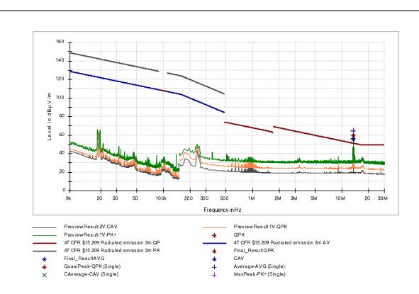
Figure 14: Chart of emissions test below 30 MHz without tag in position 1, antenna in line at 3 m, RS-232 active
