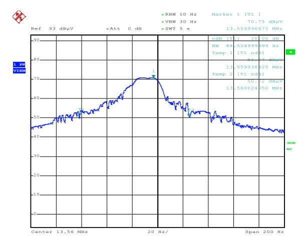
Figure 10: Chart of 20 dB bandwidth tests
