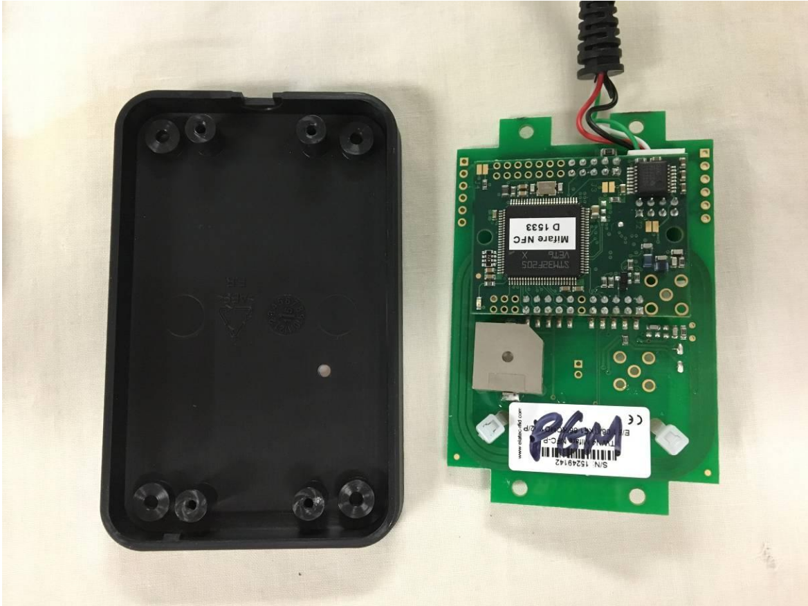
Figure 2. NFC Board Removed
