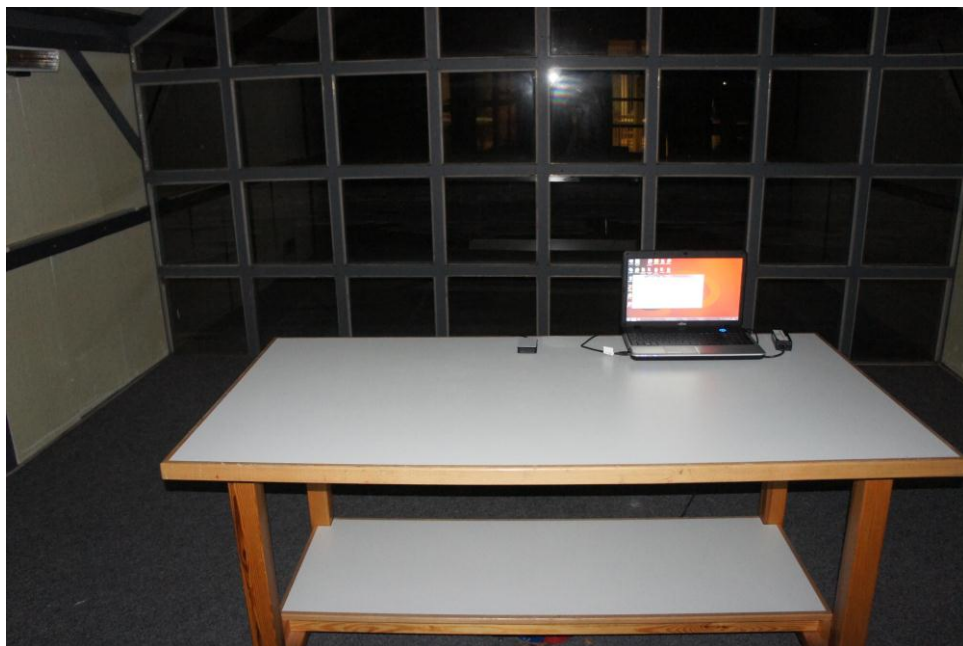
Picture 2: EUT test setup radiated emission test at open site (30MHz to 1000MHz)
