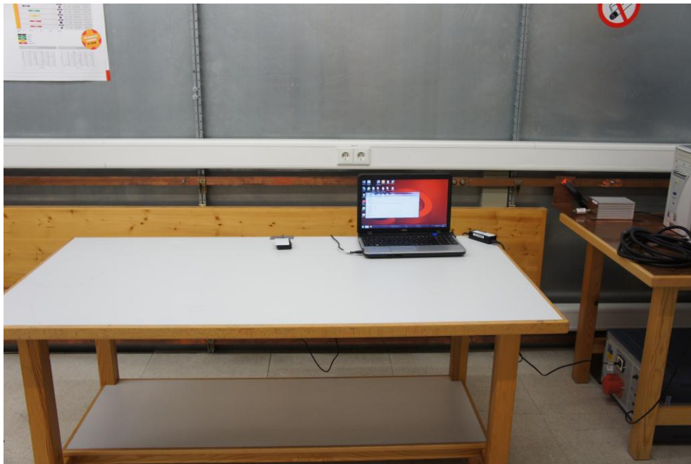
Picture 4: EUT test setup conducted emission test (front view)
