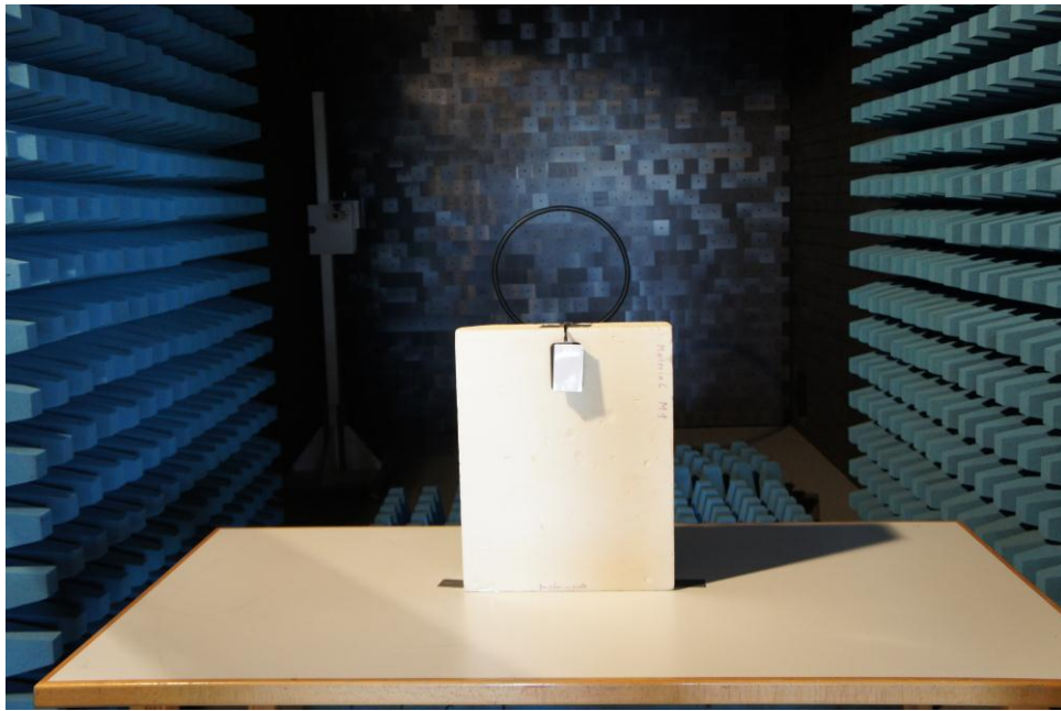
Picture 1: EUT test setup radiated emission With pre-measurements was the worst case test setup determined (9kHz to 30MHz)
