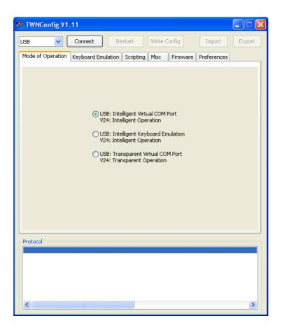
Depending on the physical interface of the TWN3 transponder reader, choose the appropriate port in the top left combo box. Click the "Connect"-button.
