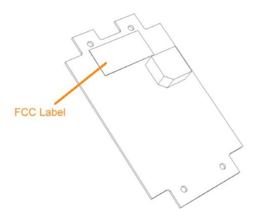
Where the FCC ID of the RFID device is not visible from the outside of the host device into which the RFID device is installed, an auxiliary label is to be affixed onto the host device referring to the RFID device inside the host; such as
