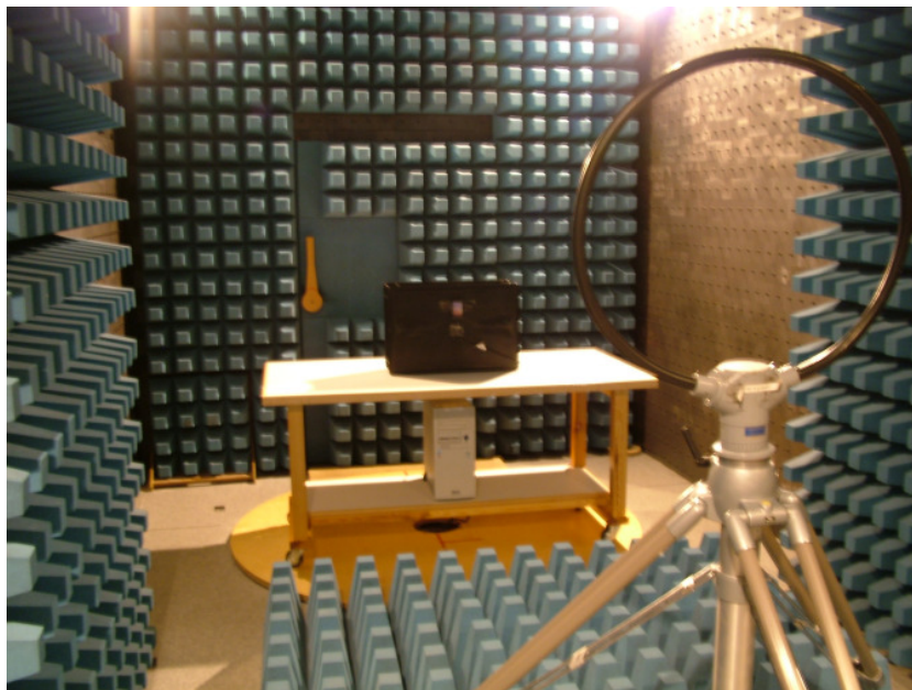
Picture 1-4: Occupied bandwidth test setup
