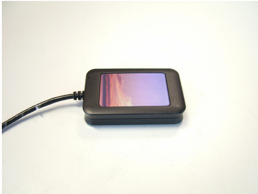
Picture 1-1: TWN3 Reader Multitag (TWN3MT) top side
