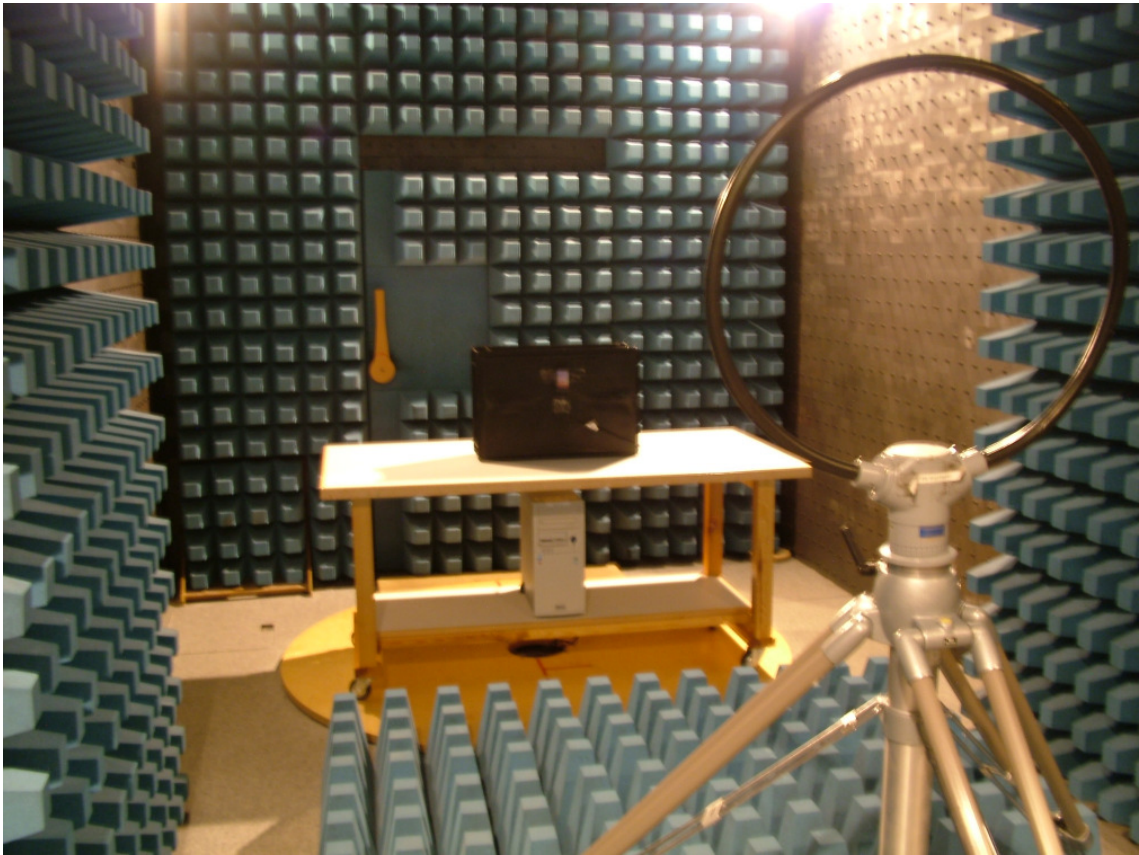
Picture 1.4: Occupied bandwidth test setup
