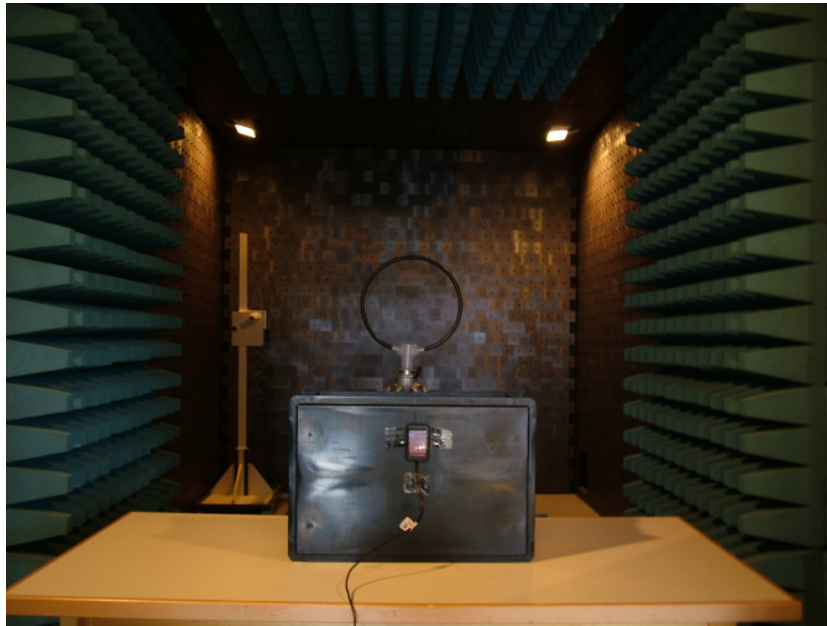
Picture 1-5: Occupied bandwidth setup
