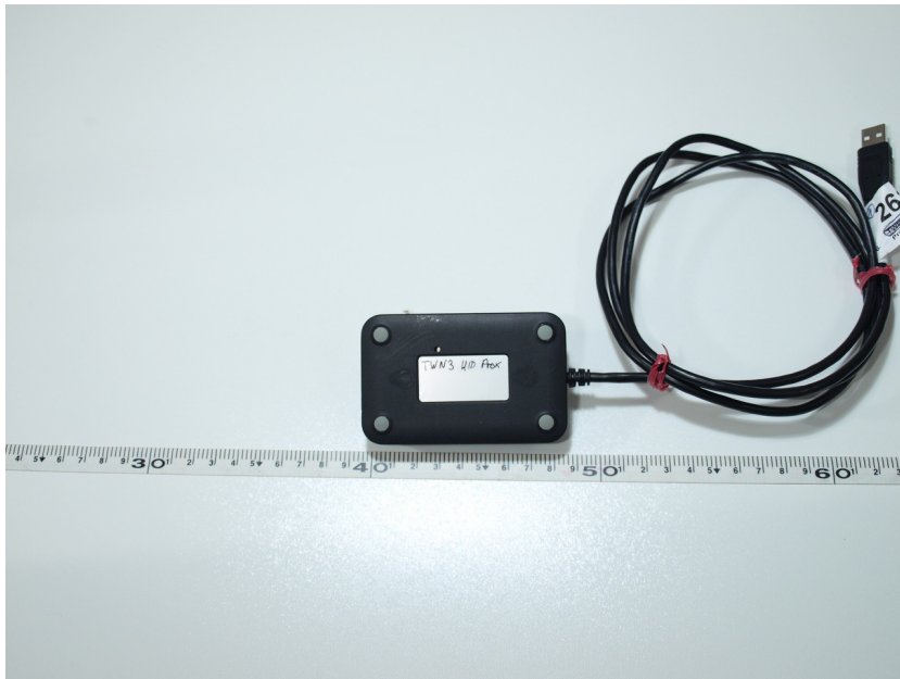
Picture 1-2: TWN3 Reader HID Prox (TWN3LF) bottom side
