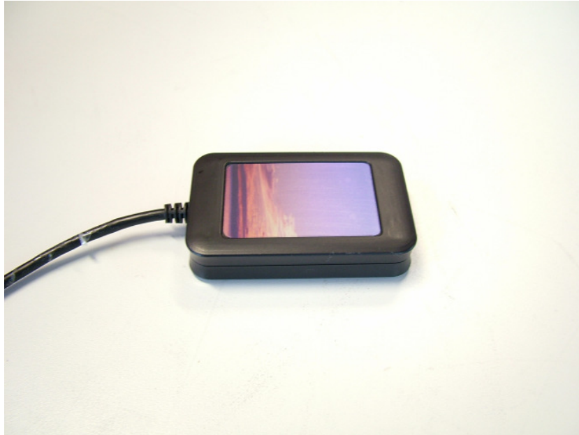
Picture 1-1: TWN3 Reader HID Prox (TWN3LF) top side
