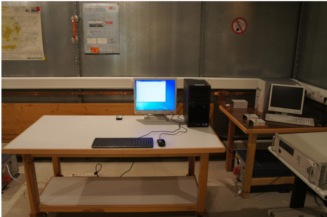
Picture 3: Test setup conducted emission (front view)
