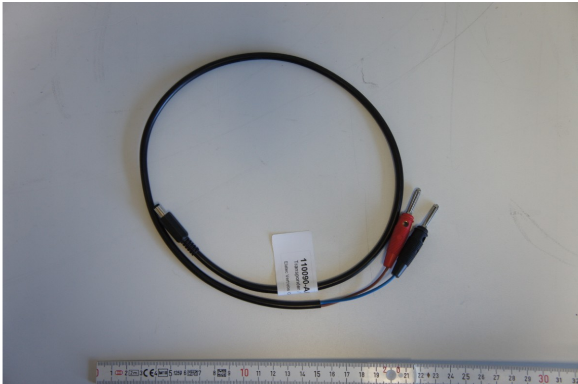
Picture 5: Power supply cable for EUT with serial connector
