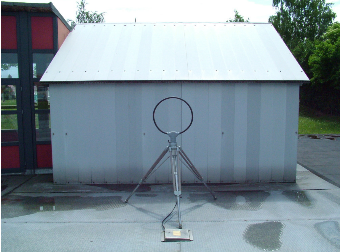
Picture 1.1: Loop antenna on open site 3m for spectrum mask and radiated emission test
