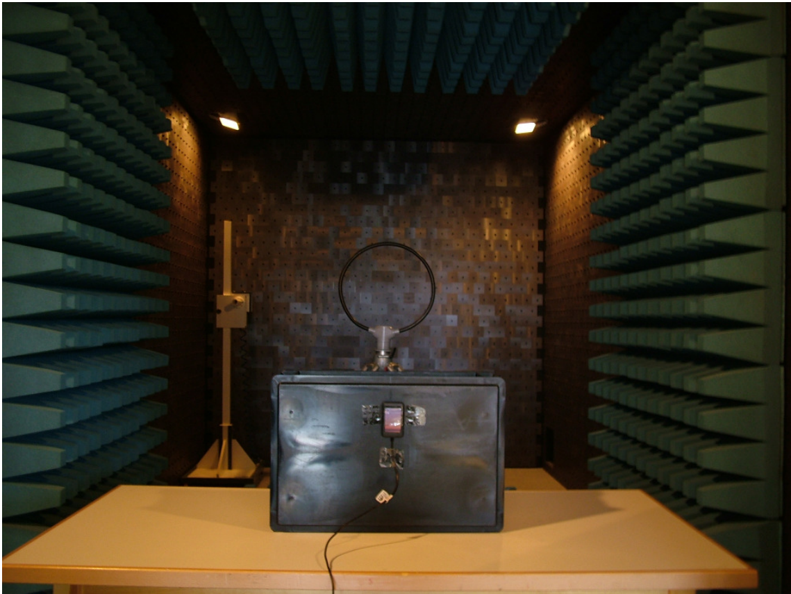
Picture 1.5: Occupied bandwidth setup
