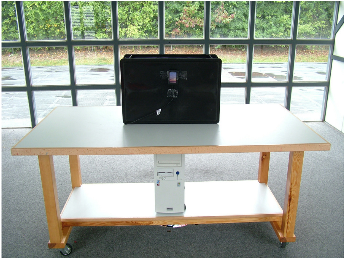
Picture 1.2: EUT test setup open site for spectrum mask and radiated emission test
