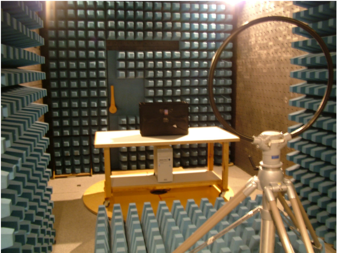
Picture 1.4: Occupied bandwidth test setup
