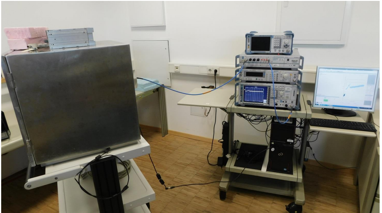
Picture 9: Conducted measurements
