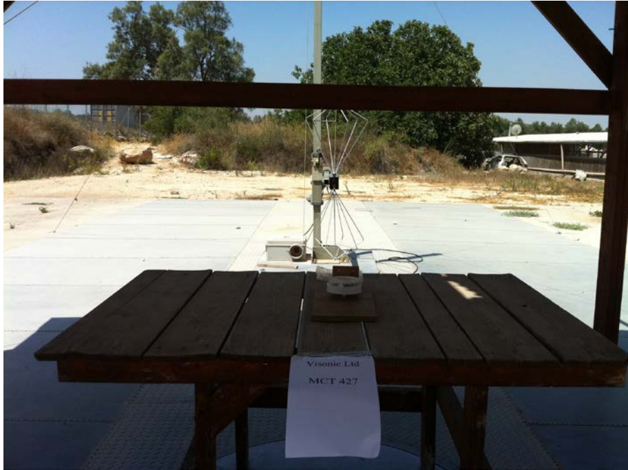
Figure 8. Radiated Emission Test Standby/Receive Mode- MCT-427 SMA
