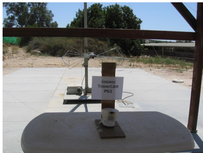
Figure 3. Radiated Emission Test
