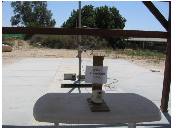
Figure 2. Radiated Emission Test
