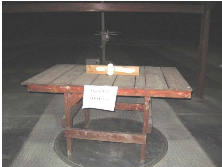
Figure 2. Spurious Radiated Emission Setup
