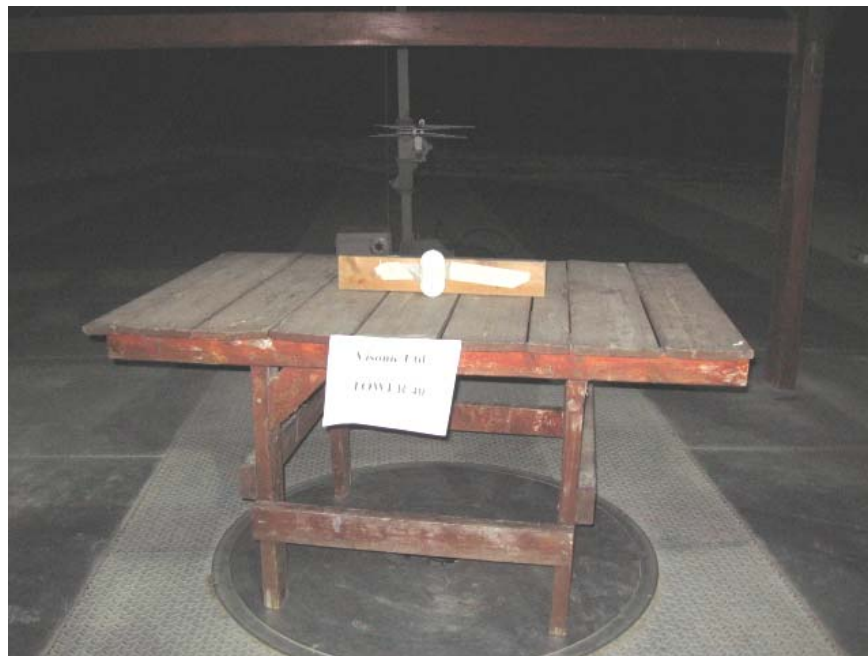
Figure 5. Field Strength and Spurious Radiated Emission Setup
