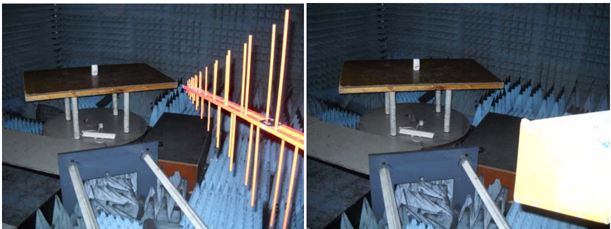
Photograph 8.1.1 Setup for radiated emission measurements
