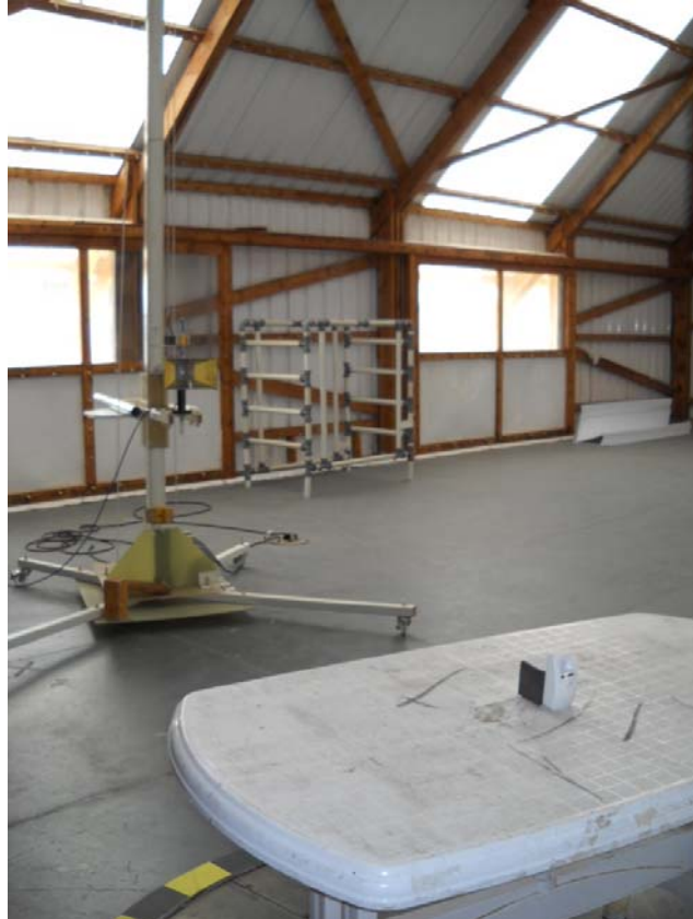
Photograph No.4 Setup for spurious emission field strength measurements at the OATS above 1000 MHz
