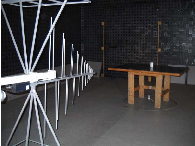
Photograph No.2 Setup for carrier field strength, spurious emission field strength measurements in the anechoic chamber in 30 – 1000 MHz range
