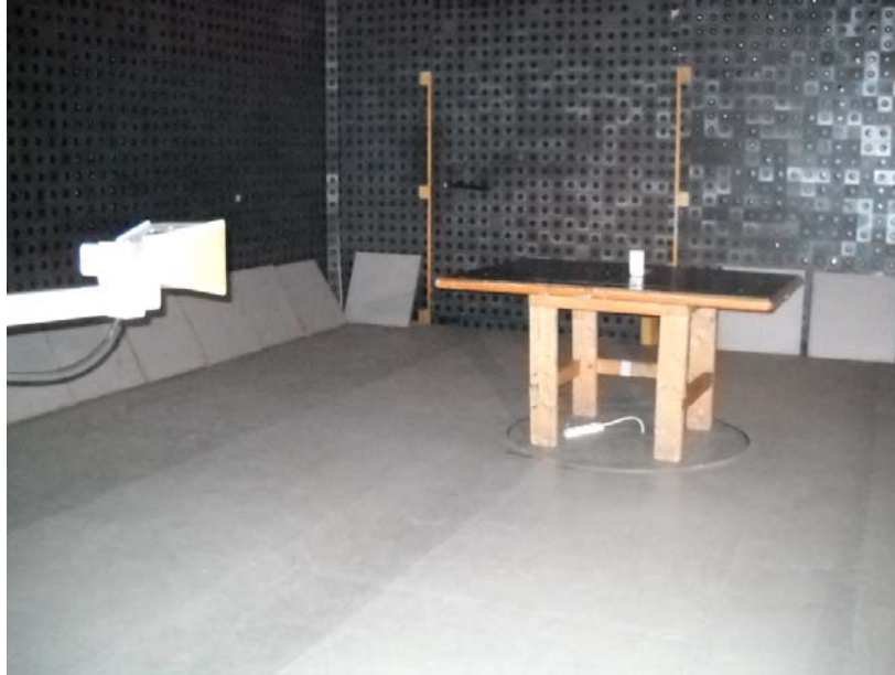
Photograph No.3 Setup for spurious emission field strength measurements in the anechoic chamber above 1000 MHz
