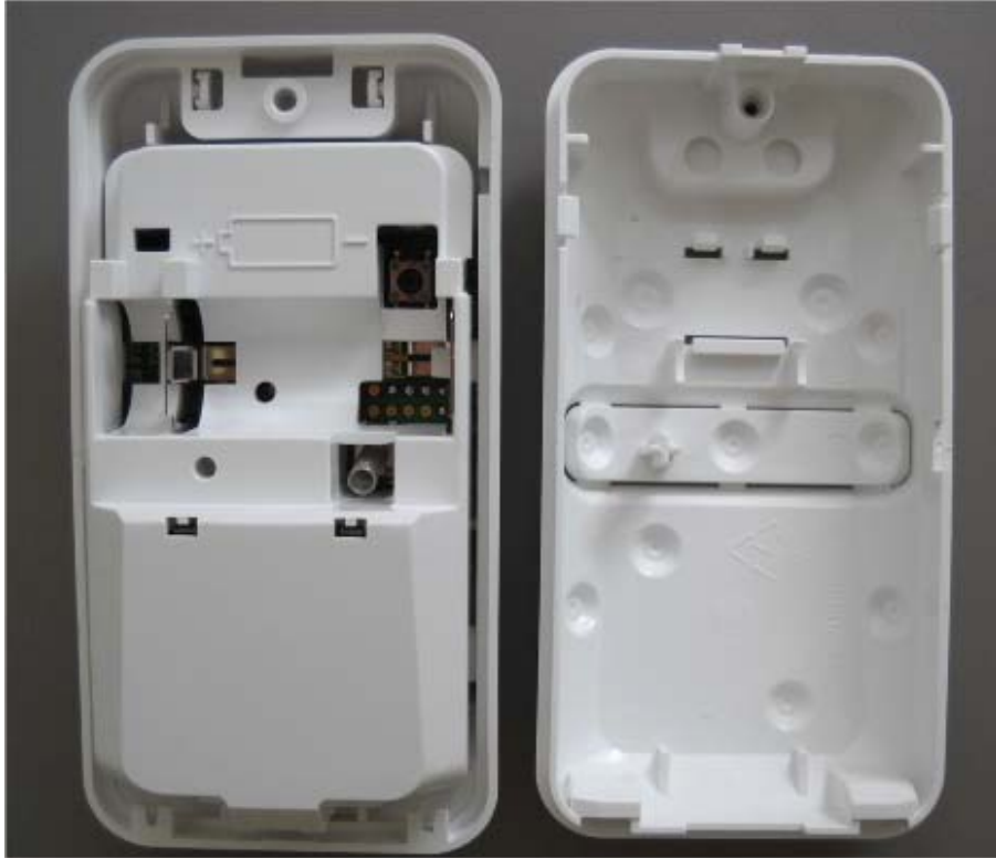
Photograph No.1 “Tower-30 AM PG2” PIR detector internal view
