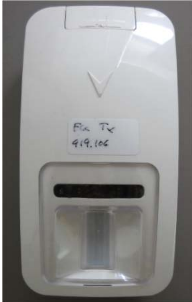
Photograph No.1 "Tower-30 AM PG2" PIR detector front view
